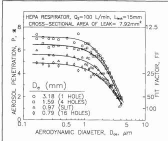
FIGURE 8. Aerosol penetration dependence on effective leak diameter
