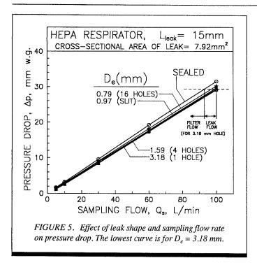
Figures 5 and 6 had the artificial leaks attached, resulting in a smaller filtration area and a slightly higher pressure drop than in the previous tests.
