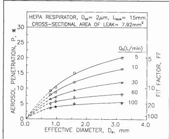
FIGURE 9. Effect of leak shape on the penetration of 2-µm aerosol particles
