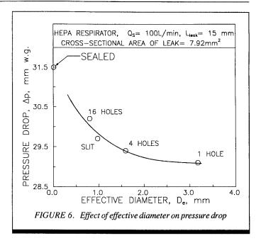
The authors conclude from this that the shape of a leak of given cross-sectional area affects the leak flow and, therefore, the penetration of aerosols.
