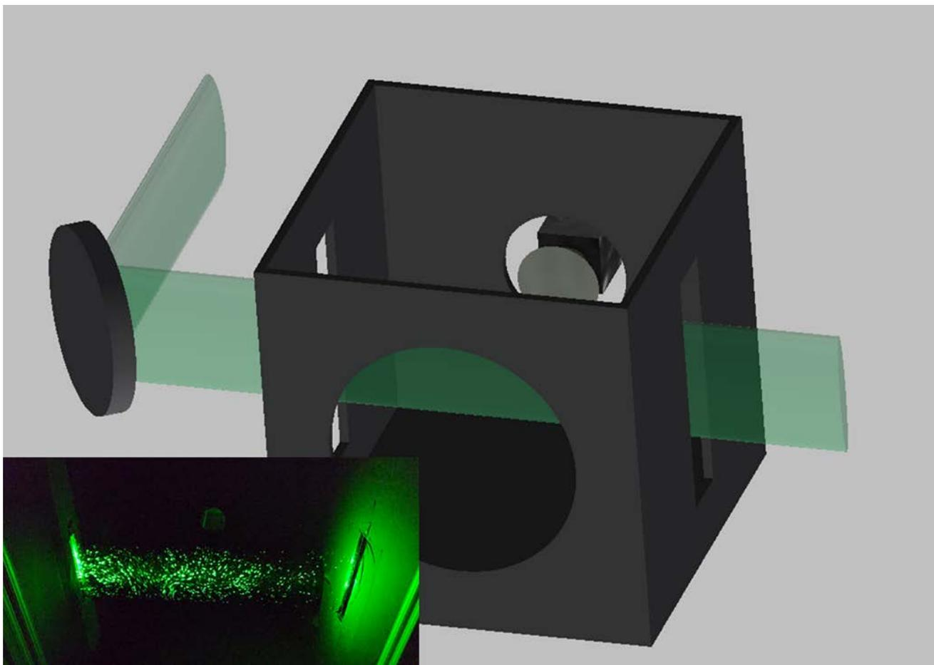
**Fig. 1. Schematic of the experimental setup.** A laser beam is expanded vertically by a cylindrical lens and shined through slits in the enclosure. The camera is located at the back of the box, a hole for the speaker in the front. The inset shows scattering for water particles from a spray bottle with the front of the box removed. Photo Credit: Martin Fischer, Duke University.
