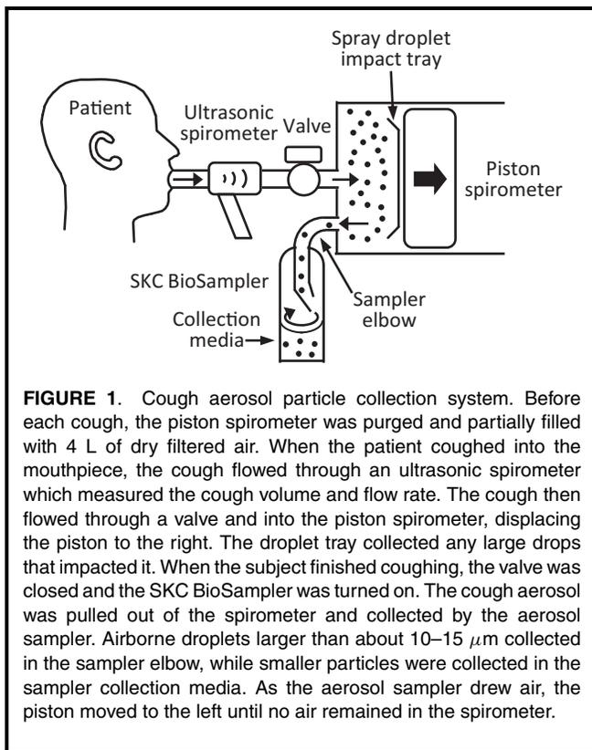
VTM to recover any virus in droplets that had impacted on the tray. The elbow was removed from the SKC BioSampler and swabbed with 3 ml of VTM to remove any virus that had impacted in the elbow during collection. The VTM collection media was removed from the SKC BioSampler and placed in a storage tube. All samples in VTM were placed on ice until the end of the day and then transported to the laboratory and stored at  $-80^{\circ}\text{C}$  until analysis.
